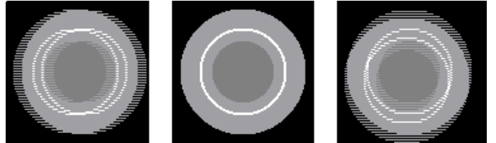
Fig. 1. Interlacing artifacts: Serration, none (progressive) and line crawl
