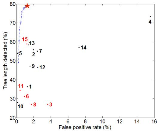
Fig. 4. Average tree length versus average false positive rate of all algorithms, with the algorithms in the semi-automated category in red. The fusion scheme ( $T_f = 2$ ) combining all 15 algorithms is indicated with  $\star$ . The blue line indicates the fusion results of including different number of algorithms, starting from 2 to all 15 algorithms.
