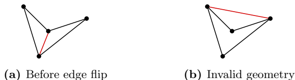
Figure 4.1: Example of an illegal flip. Flipping the red edge in Figure 4.1a produces the invalid geometry in Figure 4.1b. Edge flip is in this example not legal.
