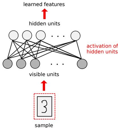
**Fig. 3.** The trained RBM can be used as a feature extractor. An input pattern is clamped to the visible neurons. The conditional probabilities of the hidden neurons to be 1 are interpreted as a new representation of the input. This new representation can serve as input to another RBM or to a different learning system.
