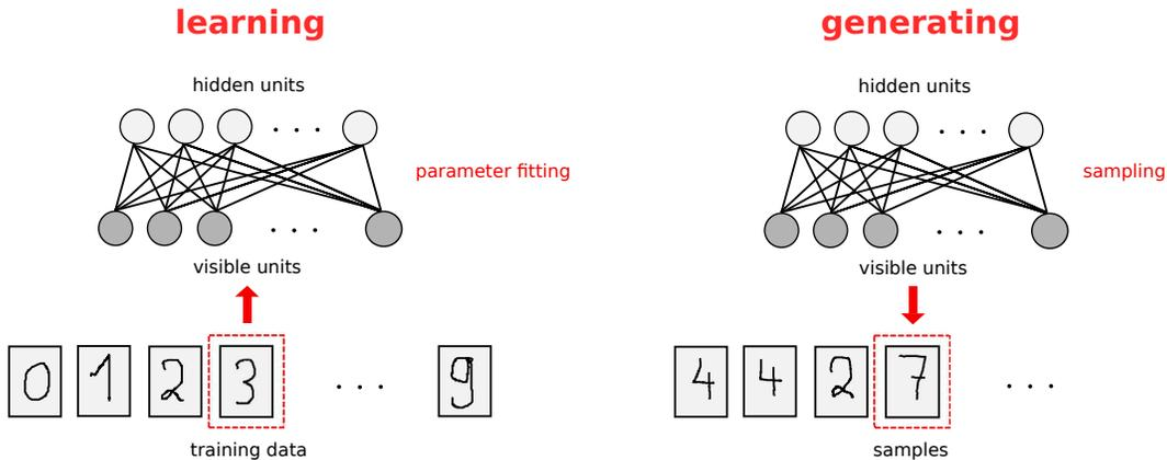
**Fig. 1.** Left: Learning an RBM corresponds to fitting its parameters such that the distribution represented by the RBM models the distribution underlying the training data, here handwritten digits. Right: After learning, the trained RBM can be used to generate samples from the learned distribution.
