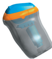
CIC shell with faceplate and electronic components
