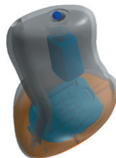
Positioning the sound exit
